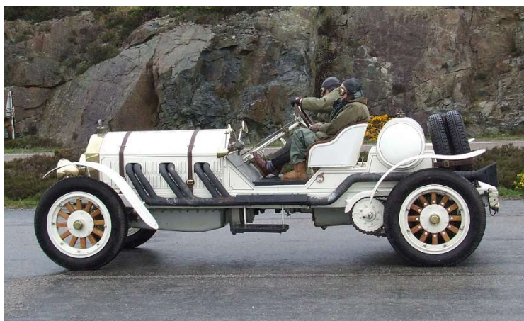
1917 La France 14 litre six cylinder engine, chain drive, brakes on rear wheels only.
